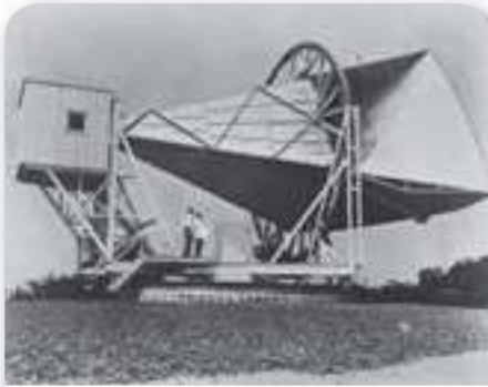
■ Figure 30.23 The cosmic background radiation was discovered by accident with this radio antenna at Bell Labs in Holmdel, New Jersey.
